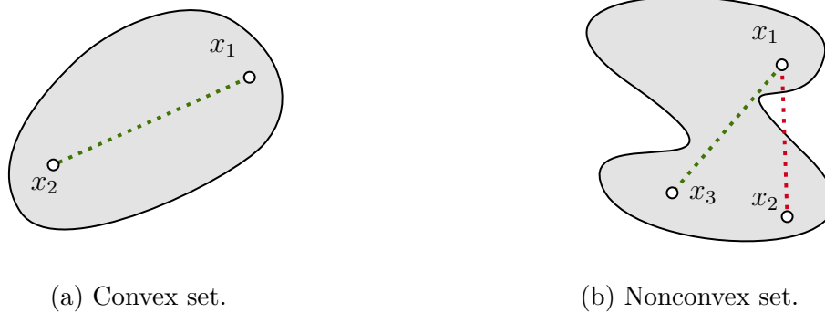
Figure 5.1 Examples of convex and nonconvex sets. (a) The oval shape is a convex set (b) The 's' shaped set is not convex, since the red line segment between x_1 and x_2 is not fully contained in the set.
